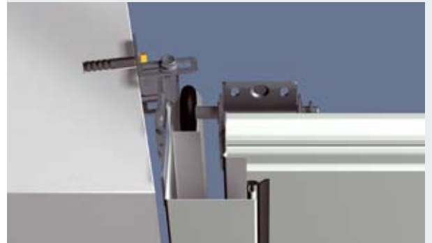
Chamfered and uneven side wall
